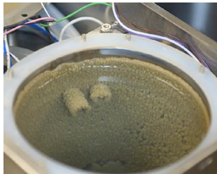
Water tank without Scale-Pro in use.*
